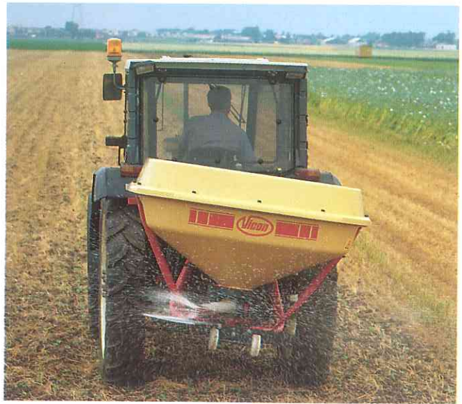
Tramline border spreading with tiltable headstock
