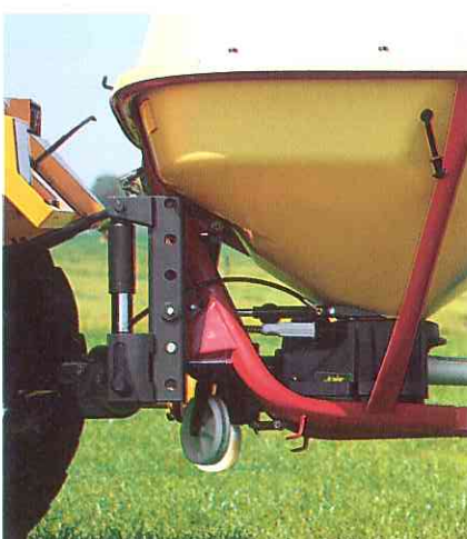
Hydraulically tiltable headstock
