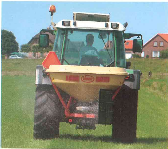
Border spreading with border spreading plate
