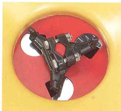
Agitator ensures even feed of the fertiliser
