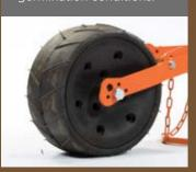
Seed Press Wheels – a range of rubber tyre seed press wheels ensure optimum seed to soil contact in advance of the soil coverer's
