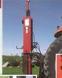
The driver is mounted on a base plate that allows the unit to tilt in two directions, making it easy to drive posts straight — even in uneven terrain.
