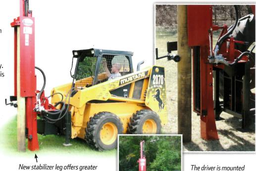
I he driver is mounted on a base plate that allows the unit to tilt in two directions, making it easy to drive posts straight—even in uneven terrain.
