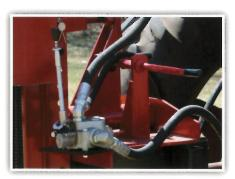
Offset controls allow the operator to stand safely to the side of the unit while posts are being driven.
