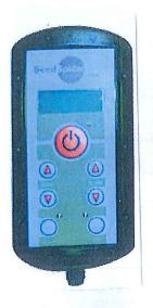
The controller has onboard diagnostics that warns the operator of malfunctions such as: driving too fast or too slow, that a specific canister has stopped working or the GPS signal has been lost.
