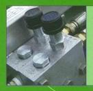
Independently adjustable cutting blade and elevator speeds
