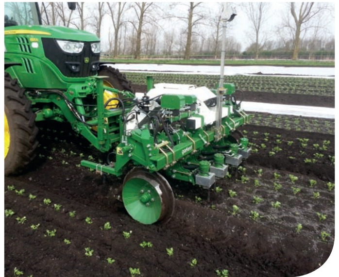
The InRow Rotors cultivate between the plants and conventional hoe tines complete the job inter row.
