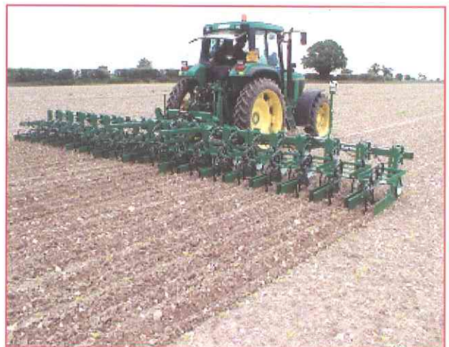
Robocrop enables large rear mounted cultivators to operate swiftly and accurately with reduced operator fatigue.
