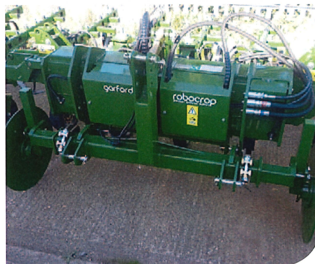
The compact hydraulic sideshift mechanism is available in Standard, Heavy Duty and Extra Heavy Duty for mounted hoes up to 18mtr
