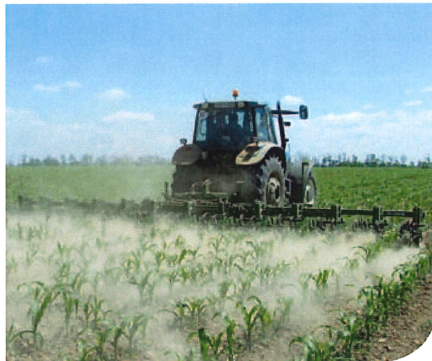
Robocrop enables large rear mounted cultivator to operate swiftly and accurately with reduced operator fatigue.
