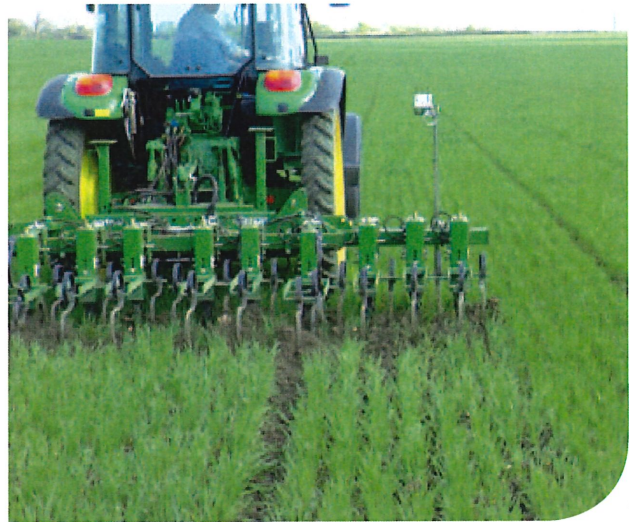
The Robocrop camera views numerous crop rows over an area of approximately 1.5mtr.sq.
