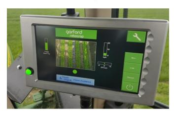
The system can also steer independently a rear mounted Robocrop Precision Guided High Speed Hoe so providing a totally hands free tractor and implement guidance operation with accuracy down to 8mm.
