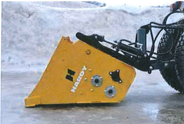
Hydraulic tilt 3 point hitch for autonomous loading (including 2 cylinders).
