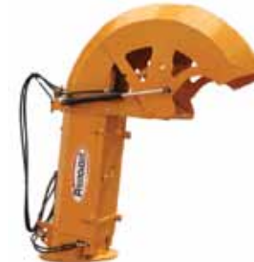
Round deflector telescopic chute Hydraulic telescopic industrial chute with rounded deflector designed for truck loading, greasable hinges and access panel.
