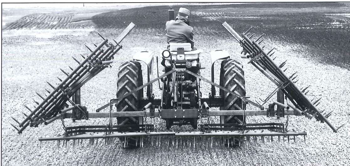
3-MD-45 Four-Section drawbar folded in transport position.
