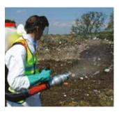
As well as being supplied as part of a complete sprayer, the Micron AU8000 spray head is also available as a conversion kit for suitable mistblowers. The kit includes connecting tubes, handle/control valve, restrictors and all attachments needed to replace a standard mistblower outlet. This kit is suitable for most types of 5HP knapsack mistblowers meeting the air flow requirements given in the specification table.
