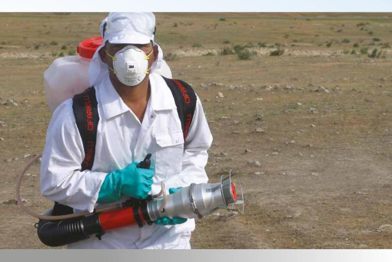
The Micron AU8000 sprayer is a highly efficient knapsack mistblower which brings the advantages of rotary atomiser technology originally developed for agricultural aircraft to ground spraying applications.
