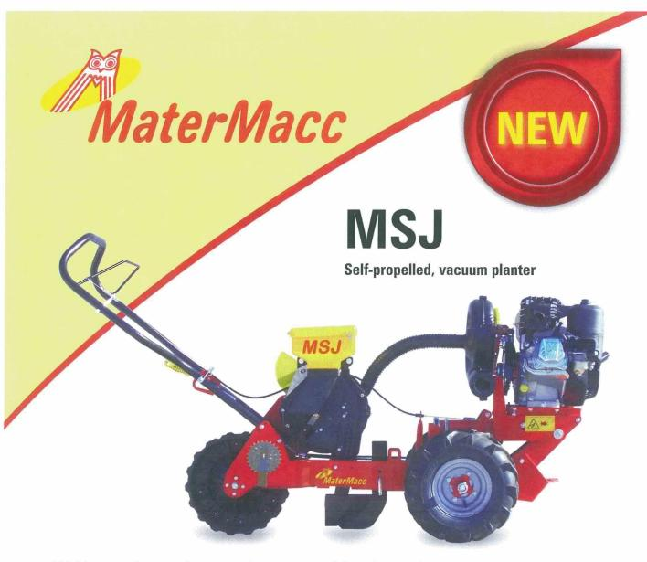
**MSJ** is a small, manually operated **vacuum precision planter**. The machine is mainly used to sow maize, chards, soy, sunflowers, rapeseed, beans, fennel, tomatoes, etc.
