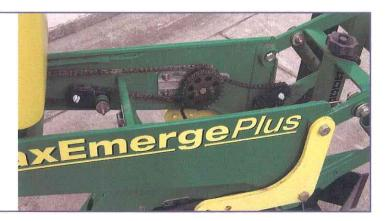
Install metering unit and snap into locked position. Use JD drive, fan, and vacuum hose.
