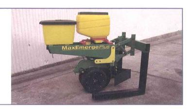
Check to see that JD drive sprocket is in correct position to accept the Matermacc
