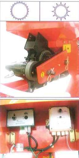
The distributor is unique. It consists of two loading cells in a different profile one for larger seed and one for small seed. The loading cell can be selected by a sideway shifting movement along the drive shaft. This system permits to change seed type very quickly.
