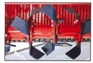
Used to bury stones, vegetable residue such as roots, harvest remains and small sticks by means of specially designed tiller blades that, in the soil, pull out the stones and throw them against the selection grill.
