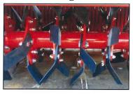
Used to fracture and bury the hard clods present in especially dry soils with high clay content by means of special tools called **blades** which, in clay soils, break up the clods and throw them against the selection grill.
