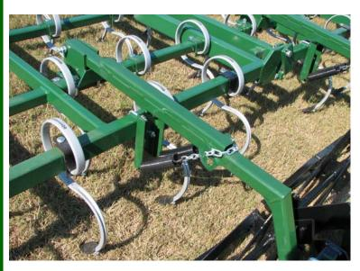
Maximum soil stirring action and excellent trash clearance is provided by the special arrangement of strong, high-quality S-tine shanks on the implement. Shanks constructed from 3/8" x 1 1/4" spring steel with 16" mounting height. Long-wearing 1/4 x 2 3/4 shares and standard.
