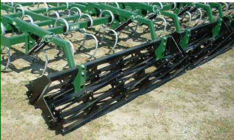
Heavy-duty crumbler attachments are hinged to middle of mainframe for reduced stress when lifting. Spiral strips are made of 1/4" x 1 1/4" C1045 carbon steel for toughness and long wear. Re-enforcement plates of same type of material. Special linkage are design permits crumblers to have more floating action for increased performance on unlevel soils. Equipped with regreaseable Tri-Ply sealed bearings.
