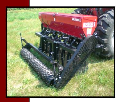
The Seed Metering System of the Valu-Drill is driven by the rear cultipacker wheels.
