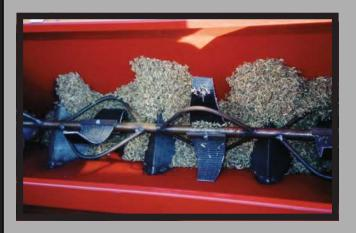
Our Optional, Patented "Positive Feed Agitator System" is designed to plant Native (Warm Season Grasses) This system is available in a second box, mounted alongside the standard Primary Seedbox. Units with box a Primary and a Warm Season Grass Box will plant virtually any seed variety wanted.
