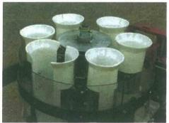
**PLANT CUPS** Six large non-stick hinged plant cups are activated with a cam. Opening each their entire length as they pass over the chute, which helps prevent plants from hanging up. Capable of setting tall plants.
