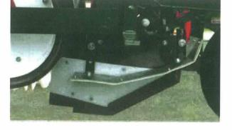
**RUBBER PACKING WHEELS** Designed to pack soil firmly around each plant.
