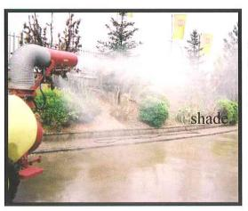
It also features a hydraulic tilt cylinder that can angle the spout from  $+80^{\circ}$  to  $-10^{\circ}$  from vertical position. The spout in the vertical position measures 7' 3" from the wheels to the top of the cannon spout. This makes the Mercury Cannon ideal for getting under an 8ft nursery
