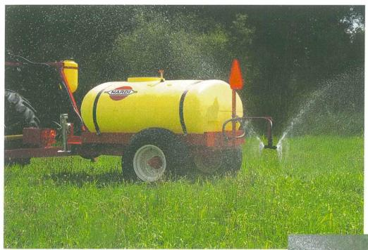
The HARDI® Giant End Nozzles provide a consistent spray pattern and droplet distribution. They are recommended for use at 20" (50 cm) nozzle spray heights.
