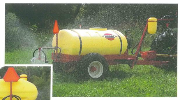
300 gallon (1100 L) and 550 gallon (2000 L) polyethylene tanks are available. The tanks are UV stabilized and very robust. They are easy to clean and feature a sump centrally located in the tank for good priming of the pump
