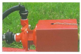
*The HYPRO centrifugal pump* is driven by the tractor PTO at 540 RPM.
