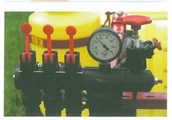
The HARDI\* BK-Manual controls feature standard 2 section controls (a third section is added with an optional hose wrap & spray gun), pressure regulator, 2-1/2" glycerin filled pressure gauge, pressure filter, and adjustable tank agitation.
