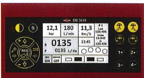
DB3610 control screen, 4 "graphic visor, easy display of all parameters: Pressure, Flow, Speed and Linked satellites, L/Ha both real and set up, Time, farms control, Valves status and Error diagnostics.
