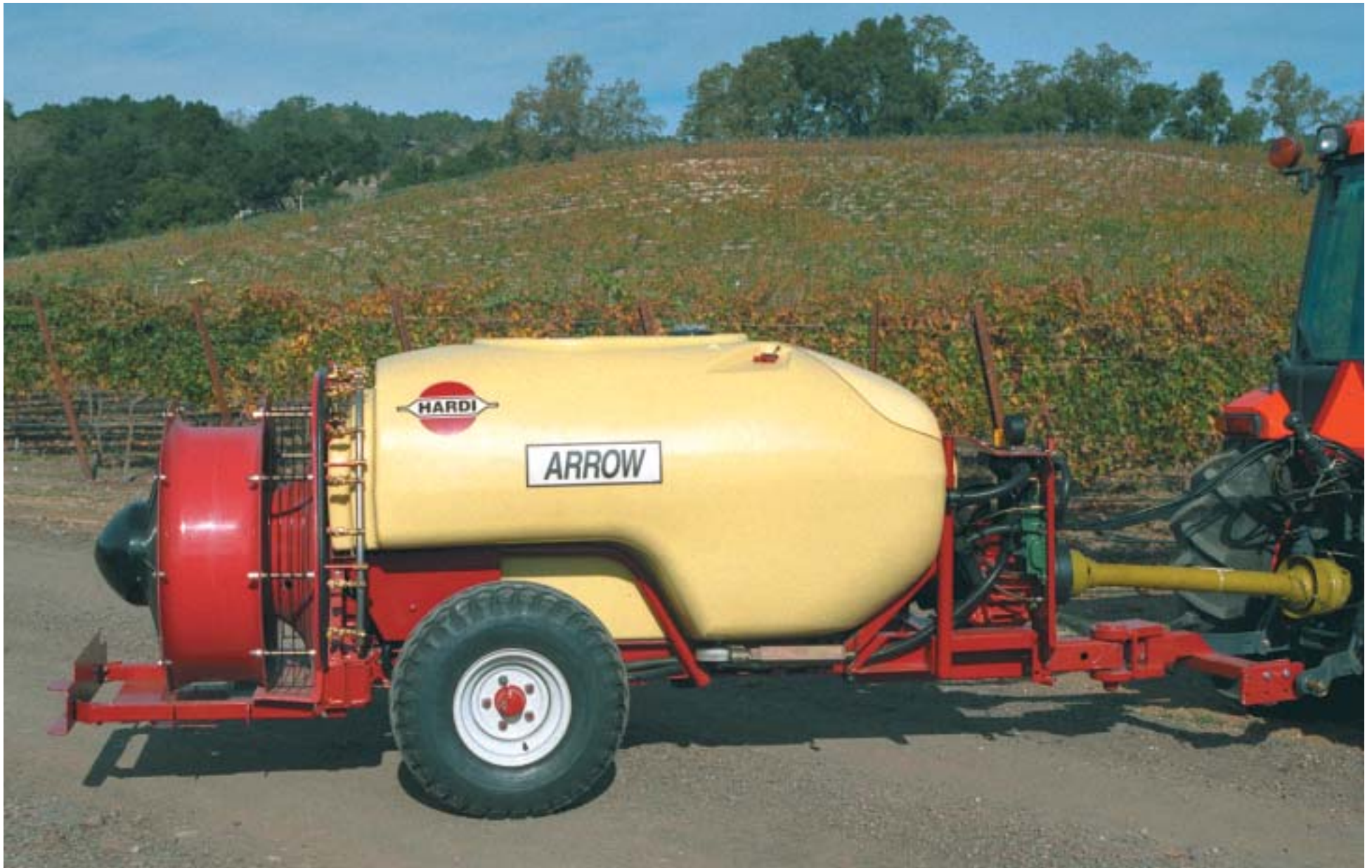
ARROW 270 with 30" Super Flow axial fan
