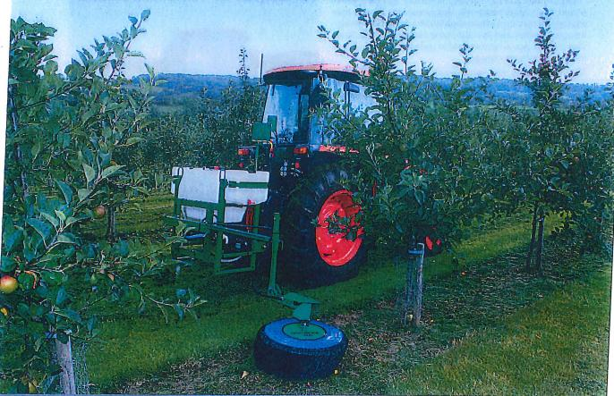
Incorporating either traditional hydraulic pressura nozzles or Micron CDA (Controlled Droplet Application) atomisers, the Undavina range of vehicle-mounted sprayers offers an efficient and targeted method of weed control round the base of vines and fruit trees.
