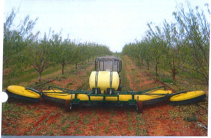
Incorporating proven Controlled Droplet Application technology, Spraydome CDA is a range of adjustable-width shielded sprayers which provide cost-effective and economical treatment of weeds in almonds, pistachios, apples, walnuts and other tree crops.
