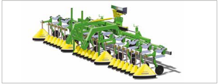
Front mounted Varidome S3 fitted with HD carriages and a combination of 100 HiFlo and 170 HiFlo shields for operation in salad onions.
