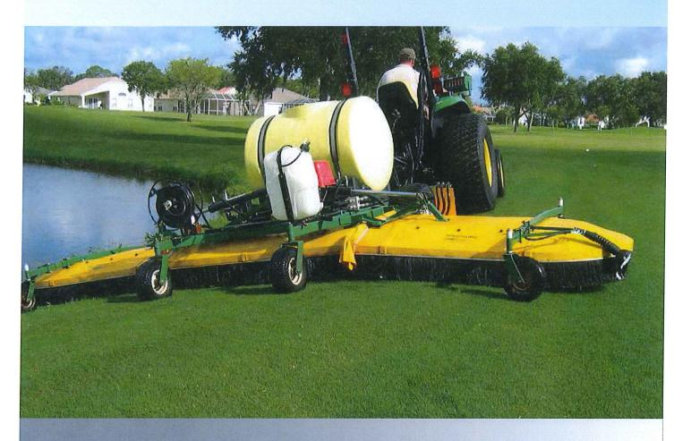
Developed in close consultation with top golf course superintendents and a result of extensive research and trials, the Spraydome T range of turf sprayers offers users increased productivity, efficient chemical usage and excellent spraying results.
