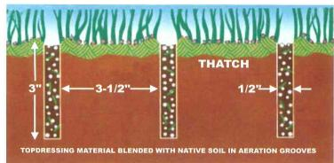
infiltration and retention, turf and root growth, nutrient absorption and organic decomposition. The one-pass design of the Earth & Turf Linear Aerator assures maximum cultivation of turf on athletic fields, golf courses and polo grounds.
