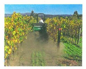
Measuring only 39 inches in width, the Vineyard Special will fit perfectly between narrow vineyard rows, yet carries 1 cubic yard of topdressing. With optional light material sides, it can carry an impressive 2 cubic yards (maximum load weight 3,000 lbs.) to keep unproductive loading times to a minimum.
