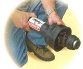
New automatic PTO clutch with 50 hour greaseable bearings eliminates shear pins. Auto latch collar remains open allowing full hand use for connecting PTO. Collar stays open until collar is installed to full positon on PTO shaft.
