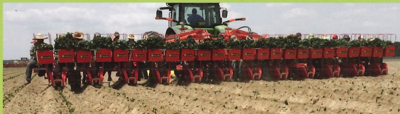
12 row/24 person FoxDrive model planting sweet potatoes at Edmondson Farms in Vardaman, Mississippi
