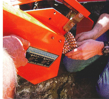
easy-to-change cogs for plant-to-plant spacing (standard)
