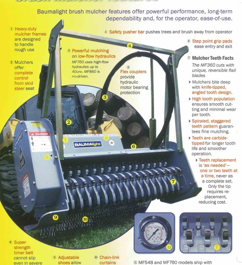
pressure gauges to monitor load. This
