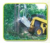
Recommended for: high performance brush cutting on high-flow hydraulics of up to 40<sub>GPM</sub>. The MF760 is a perfect fit for the midsize or largest skid steers available.
