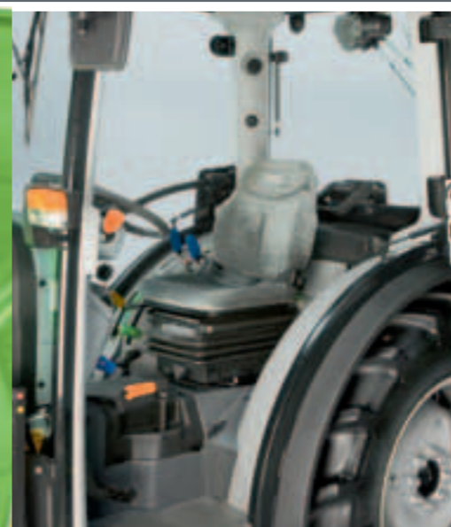
Mechanical or air-sprung comfort seat.
