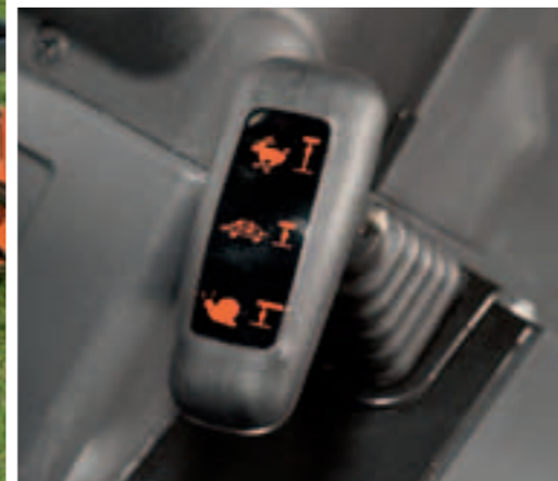
Three groups are available for up to 45 different working speeds.
