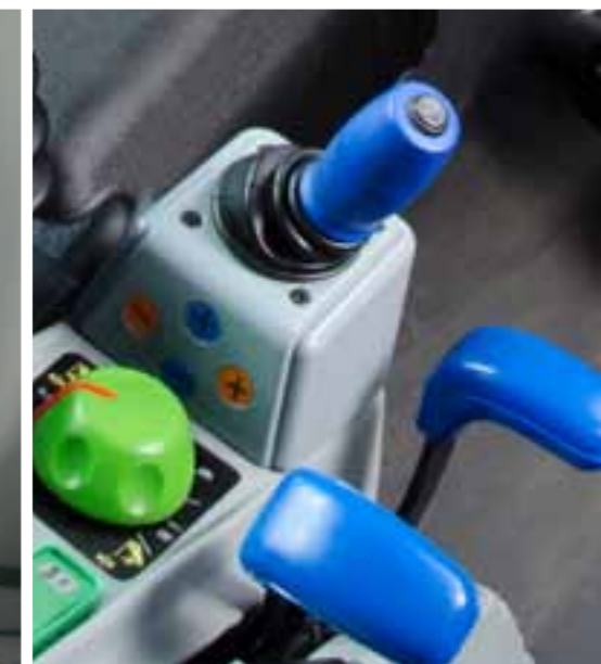
Joystick operation of the additional remote valves upon request.
