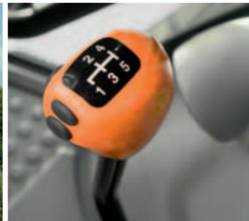
The Powershift stages are shifted conveniently with the press of a button in the shifting lever.
