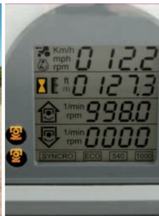
The activated PTO speed is shown on the display.
